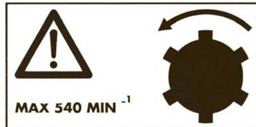
Figure 5.1 Speed and direction of rotation of PTO shaft
